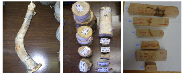
Figure 1: From left: picture of the subject tree branch sample; all sample disks; final samples cut to SilviScan specifications. The six samples selected for SilviScan analysis and subsequent calibration of local instrumentation. Birch wood samples 01-04 were cut from one Polish tree; 05—sample from 2 nd Polish tree; 06—sample from the subject tree.
