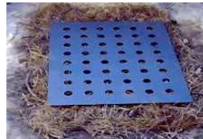
Figure 2: The position of calibration plate and combustion bed.
