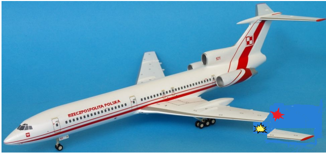
Figure 2.3: Hypothesis of explosion in the left wing.
