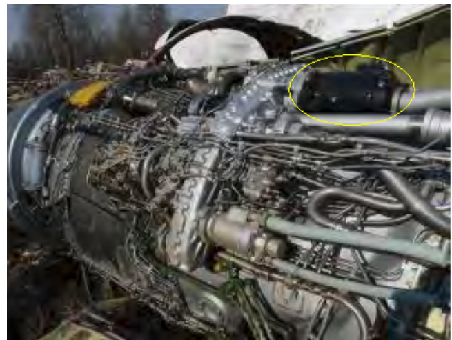
Figure 1.18: Generator GT40PCh6 on No 1 (left) D-30KU turbofan engine. Photo taken between 11 and 13 April 2010 on the crash site [15].
