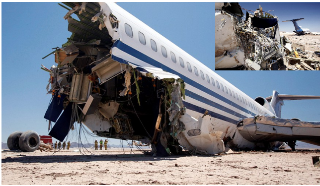
Figure 2.7: Boeing 727 after crash on Sonoran Desert with its fuselage ripped in two [47]. Compare with Fig. 2.1 .
