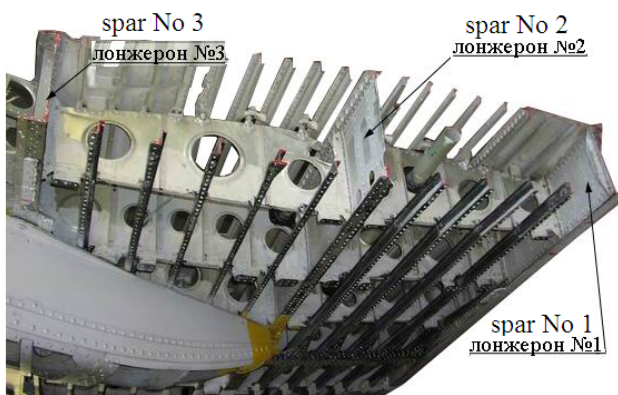
Figure 2.4: Construction of the Tu-154 wing [52].
