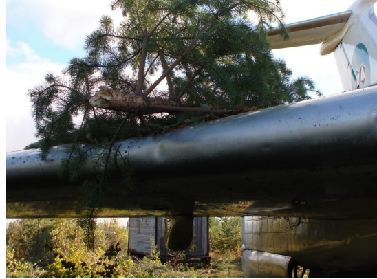
Figure 1.14: Emergency landing of the Tu-154M RA-85684 at abandoned air strip near town of Izhma on September 7, 2010. The impact was damped by the young trees which have grown since the airport was closed. The photograph shows the right wing that cut a pine tree [46].
