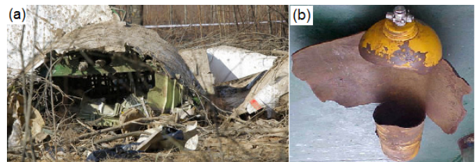
Figure 2.2: Comparison of the fuselage at the crash site on April 10, 2012 with burst gas cylinder: (a) the fuselage looks like burst from inside, the walls are split along its longitudinal axis and open to the outside ( http://krsk.sibnovosti.ru/incidents/103354-podrobnosti-krusheniya-tu-154-v-smolenskoy-oblasti ); (b) burst gas cylinder ( http://www.scubaengineer.com/scuba_cylinder_videos.htm ).
